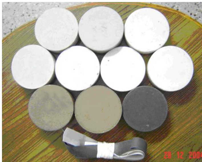
Figure 3 Virgin PTFE and its filled composite billets (before and after sintering including skiving tapes)
