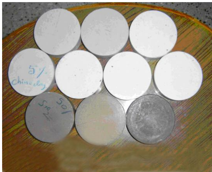
Figure 3 Virgin PTFE and its filled composite billets (before and after sintering including skiving tapes)
