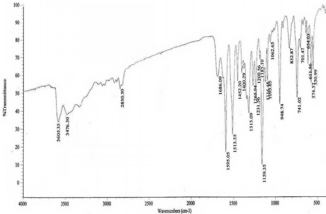
Figure 2.2 IR spectrum of p-hydroxy benzoic acid – formaldehyde oligomers
