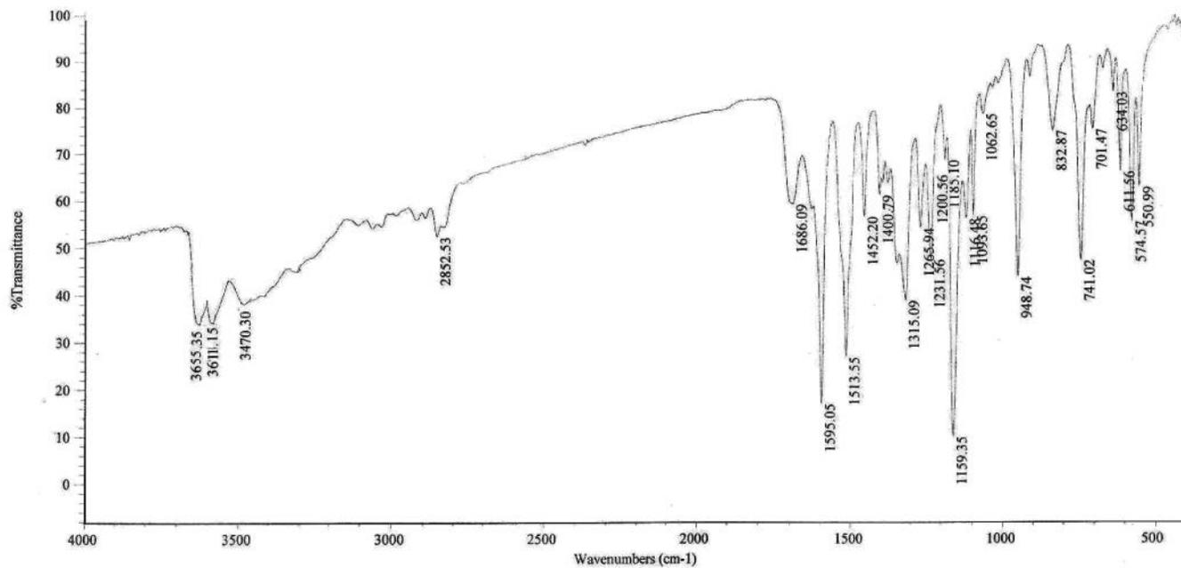
Figure 2.3 IR spectrum of Resorcilic acid – formaldehyde oligomers
