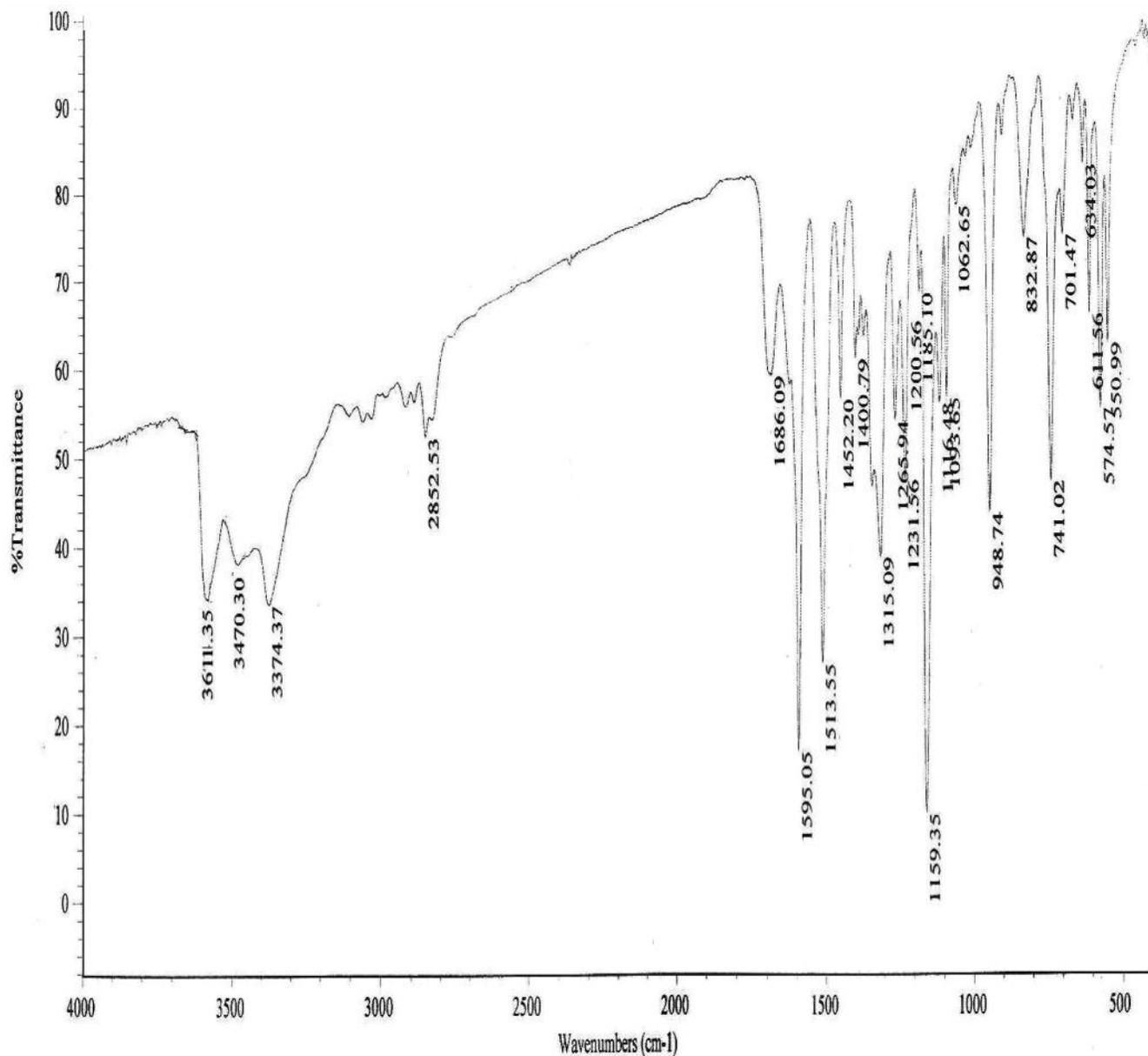
Figure 2.1 IR spectrum of Salicylic acid – formaldehyde oligomers
