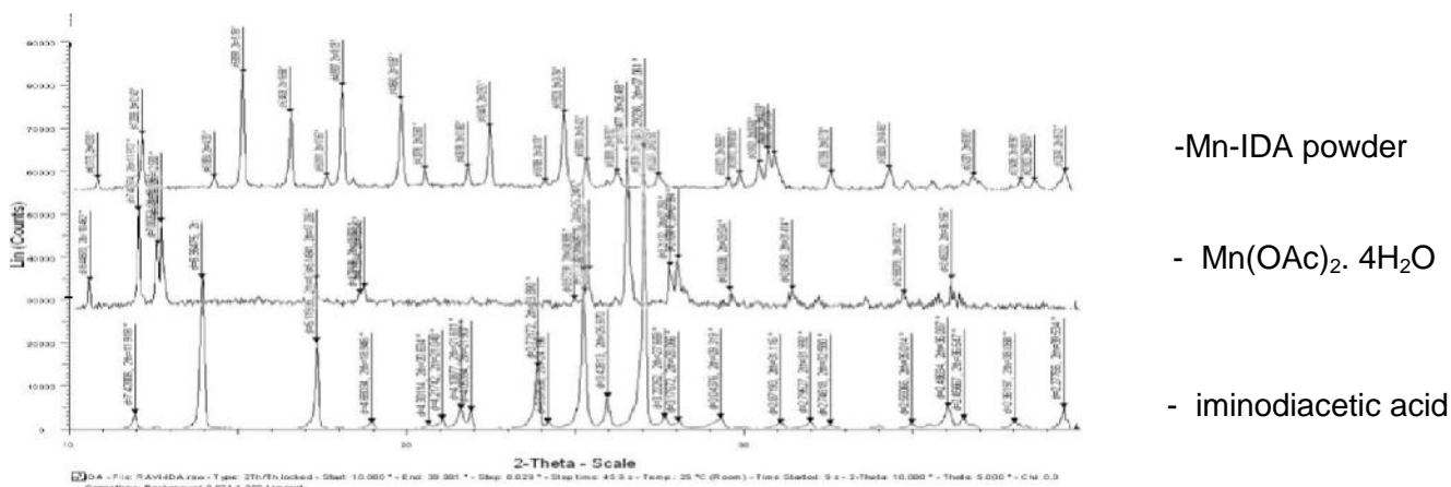
Fig.1 Comparison of XRPD patterns of starting materials iminodiacetic acid, Mn(OAc) 2 ·4H 2 O, and the Mn-IDA powder.
