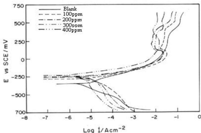
Fig. 2. Polarisation curves of brass-mm55 in natural sea water containing different concentrations of OPBT
