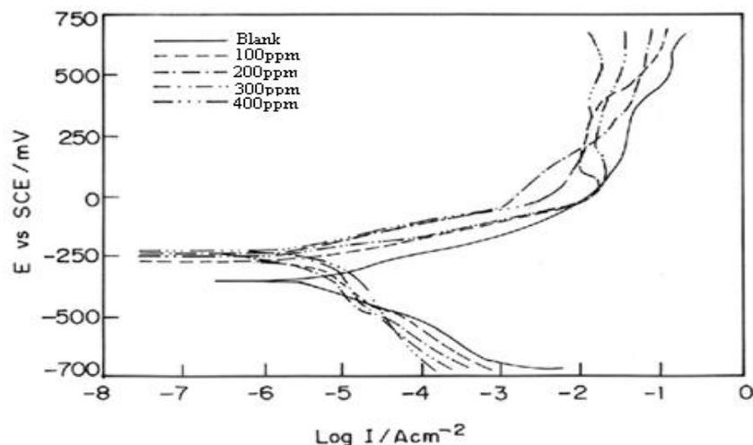
Fig. 1. Polarisation curves of brass-mm55 in natural sea water containing different concentrations of BPBT
