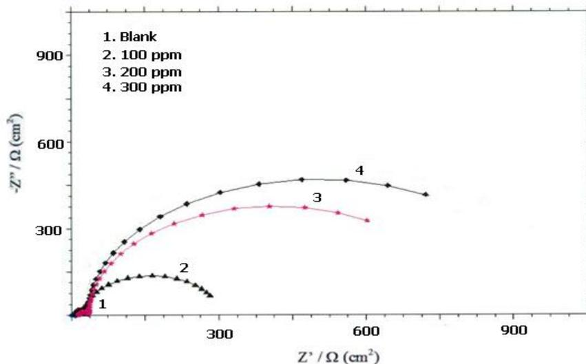
Fig. 3. Nyquist diagrams of brass-mm55 in natural sea water containing different concentrations of BPBT after immersion of 1h.
