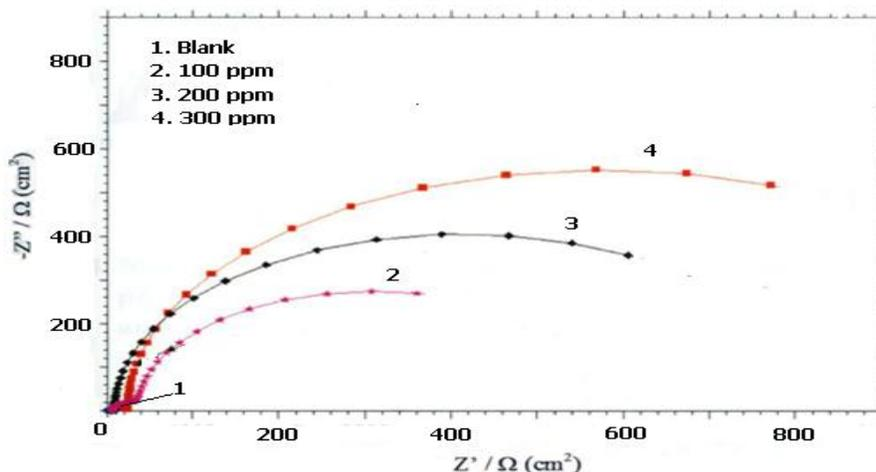
Fig. 4. Nyquist diagrams of brass-mm55 in natural sea water containing different concentrations of OPBT after immersion of 1h.
