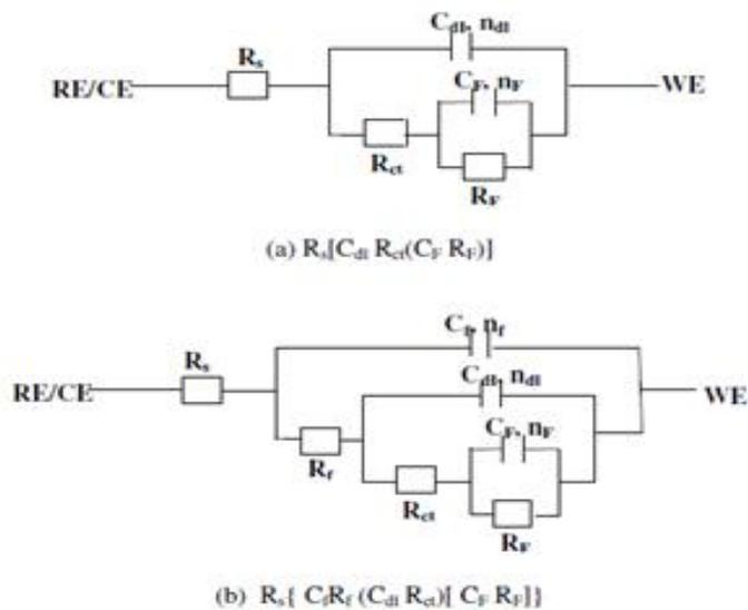
Fig. 5 Equivalent circuit diagrams for brass in (a) absence and (b) presence of inhibitors
