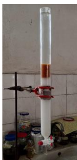
Figure 1. Chromatographic separation on open column
