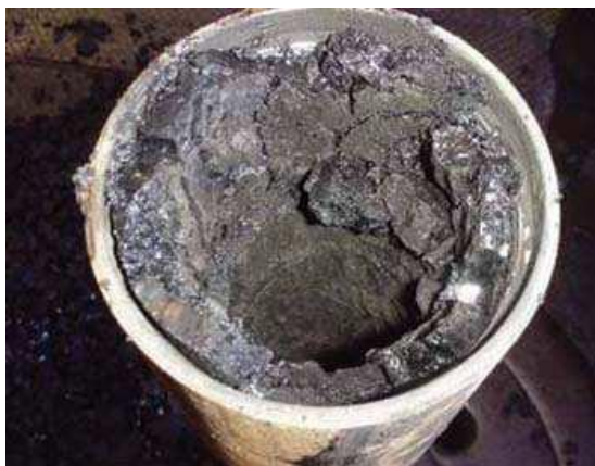
Fig. 5: Asphaltenes clogging a pipe [35]
