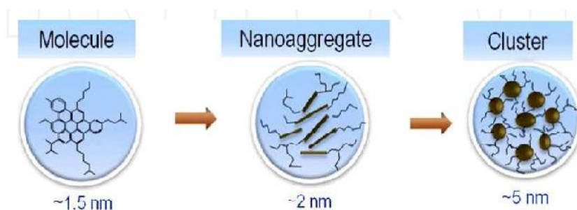
Fig. 4: Asphaltene structure according to the modified Yen model [16]
