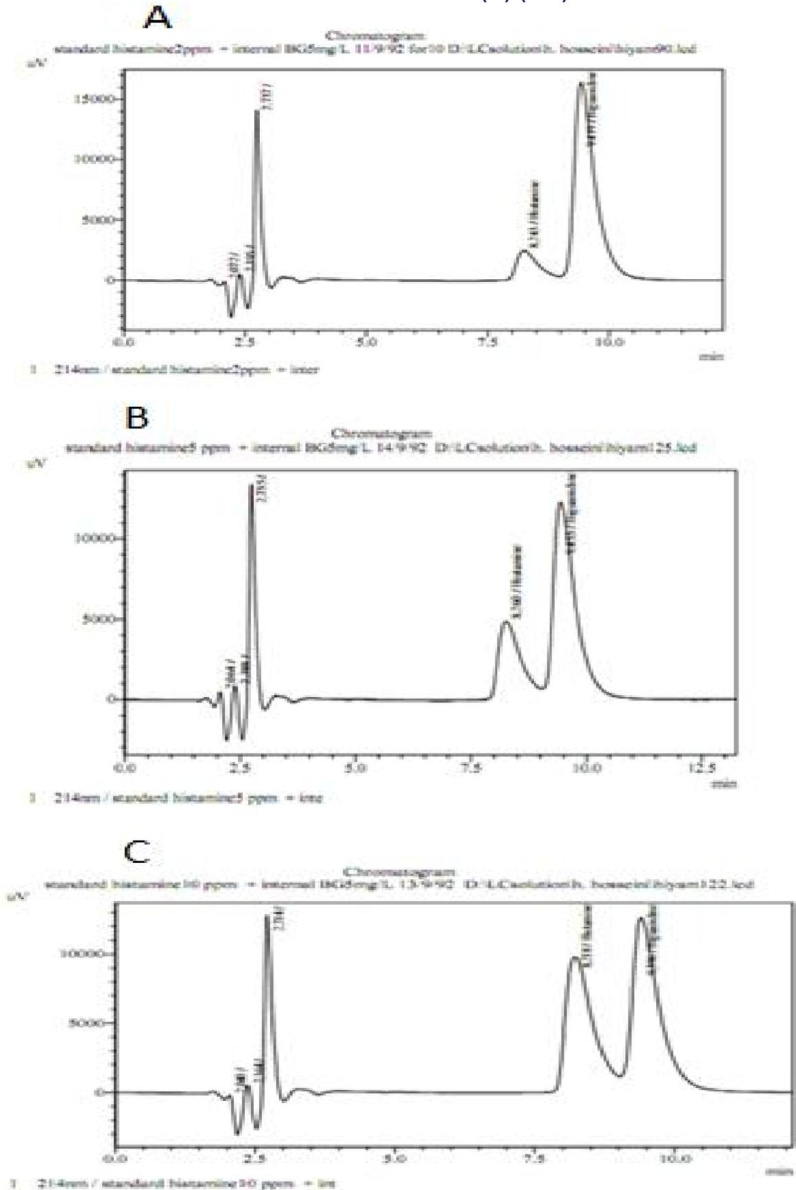
Figure 3a. HPLC chromatograms of Histamine standard A) 2ppm, B) 5ppm, C)10ppm, and 1, 1-dimethylbiguanide standard 5mg/l
