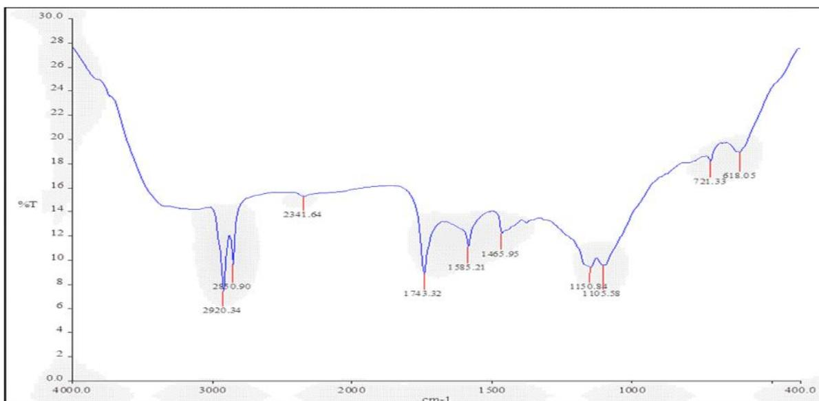
Figure 2: FTIR Spectrum of the sample PT
