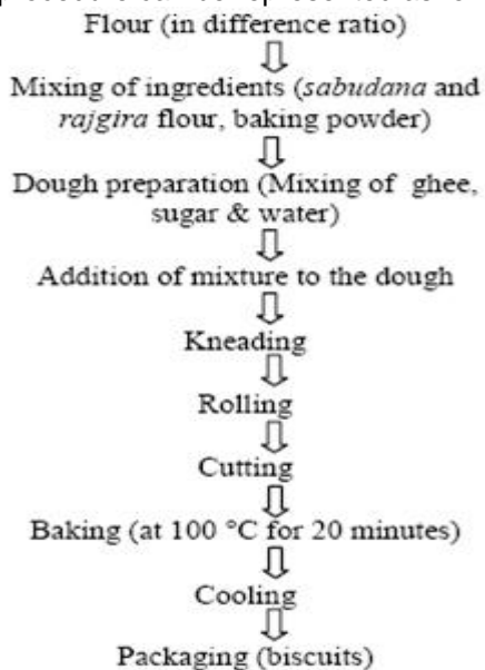
Fig : Process flow chart of Biscuit preparation
