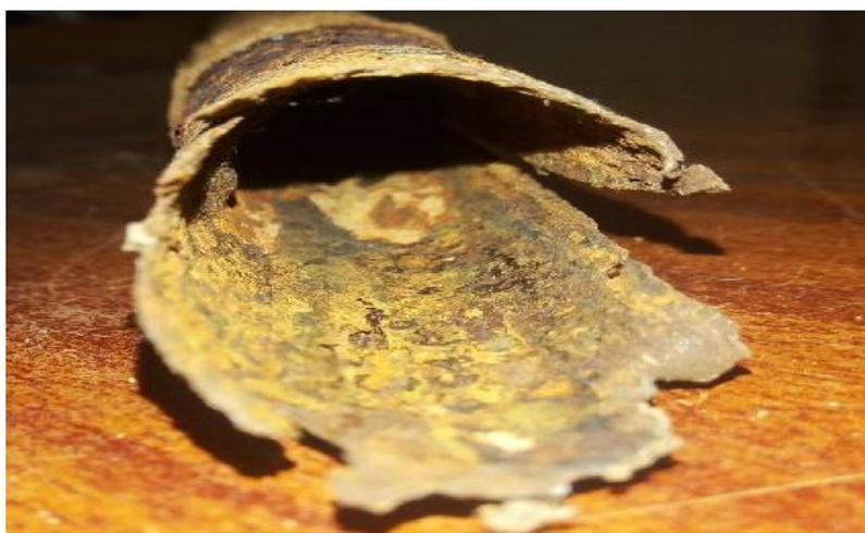
**Photo 1:** Pipe damaged by corrosion: internal view
